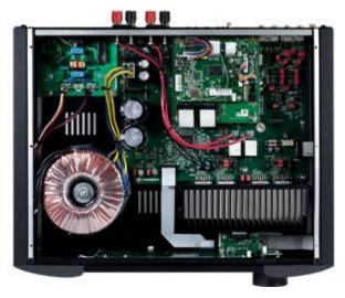
Popping off the ACE's lid reveals a jam-packed chassis. Toward the front is a heatsink that contains the four bipolar transistors used for the output stage. Rated power is 2x50W into  $8\Omega$  and 2x75W into  $4\Omega$ . Like other MOON amplifiers, the ACE operates in Class A mode to 5W, so there's no crossover distortion at levels where it could be audible.
