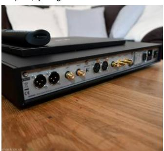
digital preamplifier so you can in theory just connect straight to power amplifiers and use the digital volume to control the levels. There is also a small switch which can raise the gain output from 2v to 6v should you require this extra level of boost. In most cases 2v will be more than enough output. One point on the connectivity is that it also features an input for an external clock to be connected which will improve the dCS Debussy's performance even further.
