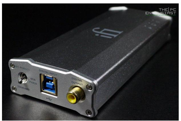
Meanwhile, at the back of the micro iDAC2 you can see the SPDIF or digital output, the USB 3.0 Type-B digital input and filter switch. iFi recommends for best sonics, with PCM music use Bit-Perfect and for DSD music use Extreme. However you also need to try the different
