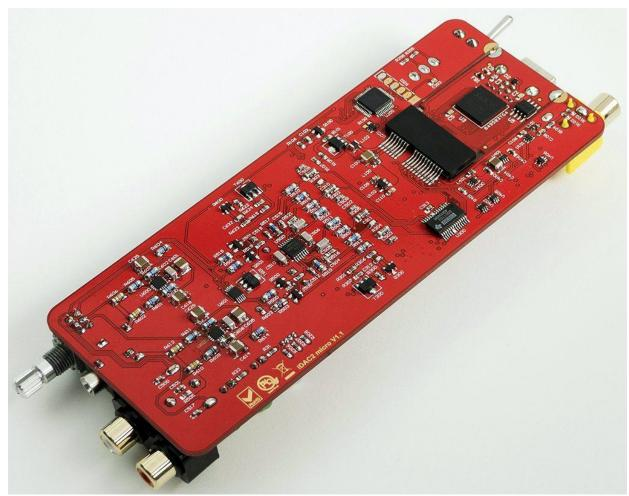
At the bottom portion of the iDAC2's PCB you can see more of the components like the Burr-Brown DSD1793 DAC chip, XMOS USB chip and more. Notice that the USB digital input section is somewhat cut-out or separated from the main PCB. I think this is to ensure that the incoming signal stays clean and noise free.
