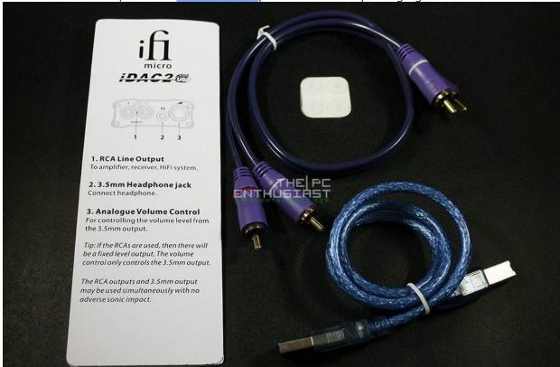
The micro iDAC2's packaging includes a reading material, an RCA interconnect, USB 3.0 to USB Type-B cable, four rubber feets and the micro iDAC2 itself. By the way, I noticed that iFi changed the rubber feets compared to the previous ones. iFi's logo is engraved on each rubber feet, but the rubber feet itself is thinner compared to the rubber feet that came with
