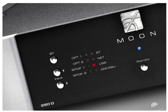
At the faceplate's far left is a column of three silver buttons: the topmost is labeled BT, for Bluetooth discovery mode; the lower two buttons are for scrolling among the various inputs. To the right of these are two columns of four red LEDs each, one for each input: Opt 1 and 2, S/PDIF 1 and 2, BT, Net, USB, AES-EBU.
