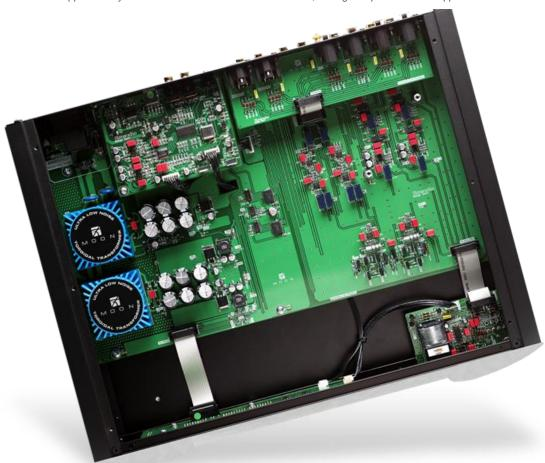
The phono section supports moving-magnet and moving-coil cartridges, and offers adjustment of the resistance, capacitance, and gain settings. The phono-circuit input replaces the pair of single-ended analog inputs labeled A3/PH, which are accompanied by a connection for the phono ground wire.
