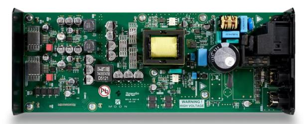
floor of -150dB at 1.0V from DC to 100kHz. M-LoVo, designed specifically for the audio signals typical of streaming DACs, is said to provide exceptionally fast, precise, stable DC voltage.
