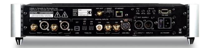
At the center of the rear panel are eight digital inputs: USB (capable of reading all resolutions up to 32-bit/384kHz PCM and DSD256), AES/EBU, S/PDIF (x3), optical (x2), and Ethernet. Wireless connectivity is supported through Wi-Fi and Bluetooth aptX. There are also MiND update and reset
