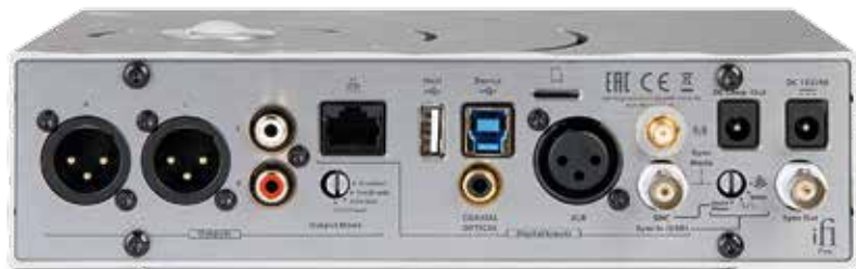
ABOVE: Digital inputs are shared across a combined coax/optical socket (S/PDIF), BNC-A and B sockets, AES/EBU (on XLR), micro SDHC and wired/wireless Ethernet. A multifunction BNC input also accepts external clock sync'ing. Balanced (XLR) and single-ended (RCA) analogue outs are fixed or variable
