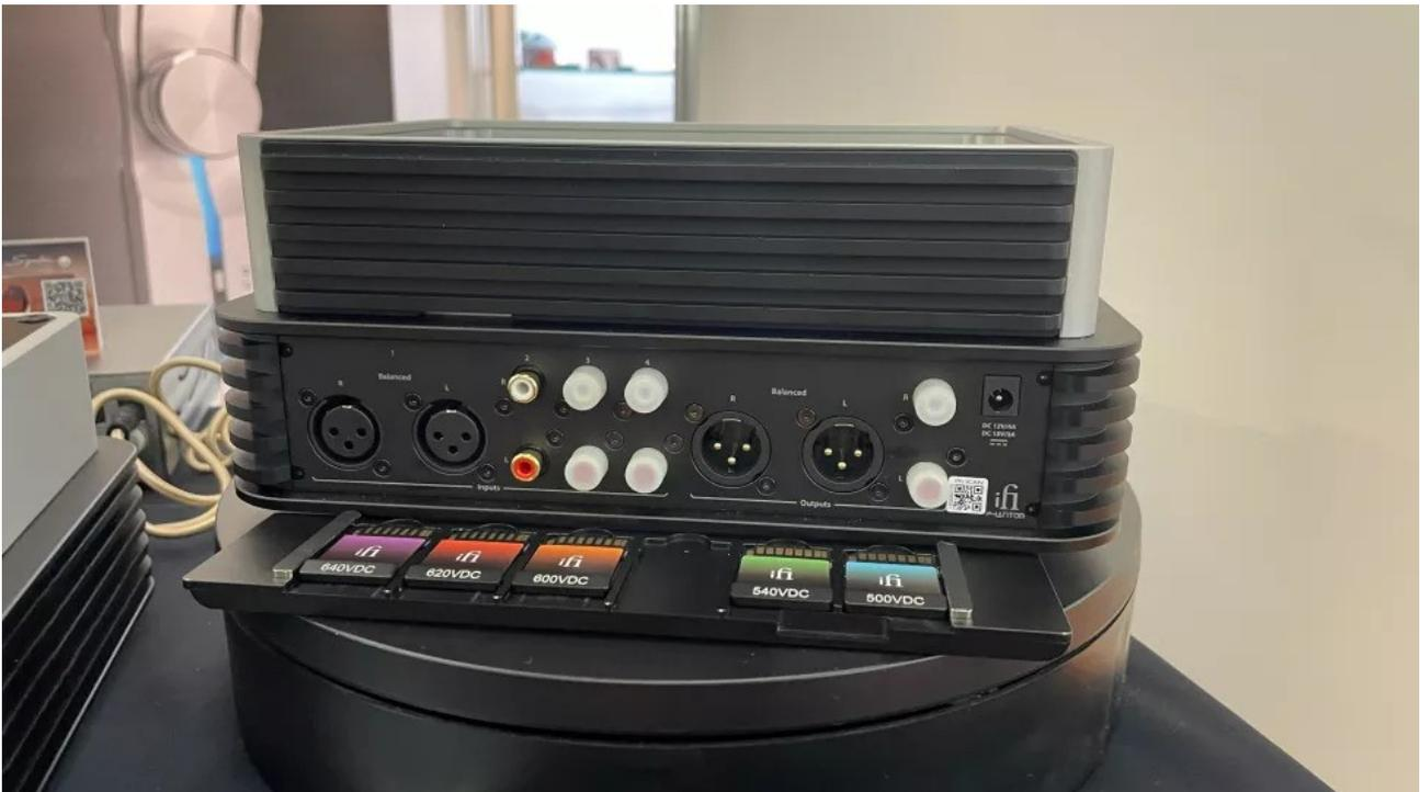
By far the most unique aspect of the Phantom is the way it “delivers the voltages that electrostatics need to perform their best.” You can't use a conventional headphone amplifier with electrostatic headphones as the voltages required to drive them are far higher than usual. So, you need a separate 'energiser' to drive them, with the correct voltage to match your specific model.
