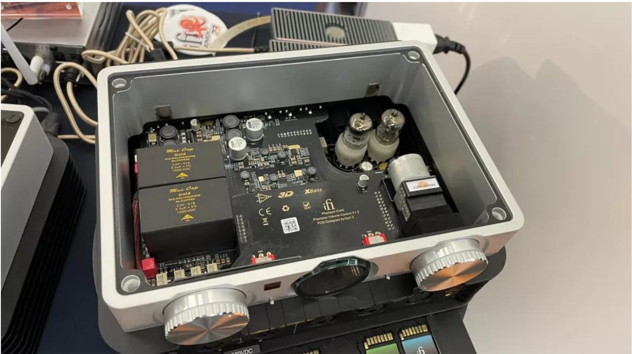
What is the iFi iCan Phantom? It's a pure analogue headphone amplifier, replacing the current flagship (Pro iCan Signature), with a brand new look and some rather clever design decisions, including a novel way of offering the correct bias voltage to match your electrostatic headphones.-
