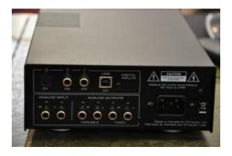
There is a 1/8" standard music player input jack at the front for the iPod generation. On the rear panel there is an Optical (TosLink) input, two S/PDIF coax inputs and a USB Type B. All of these inputs support PCM into 24 bit/192kHz. DSD (64,128,256) is only available with USB B as is PCM at rates of 32 bits/352.8 & 384kHz. A driver download is needed for DSD support which is pretty easy to set-up. There is also an analogue RCA input at the back which may be useful.
