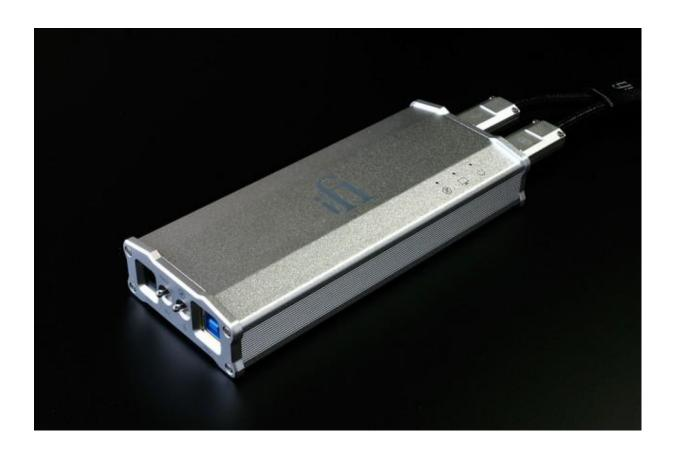
Overall build quality is similar to the micro iDAC2. Both units have aluminum outside cover. There is 9V power supply input, one USB input and two USB outputs. Thus, two separate units can be powered via iUSB3.0. For example, both HDD and DAC units may have clean electrical signals when connected to the iUSB3.0.
