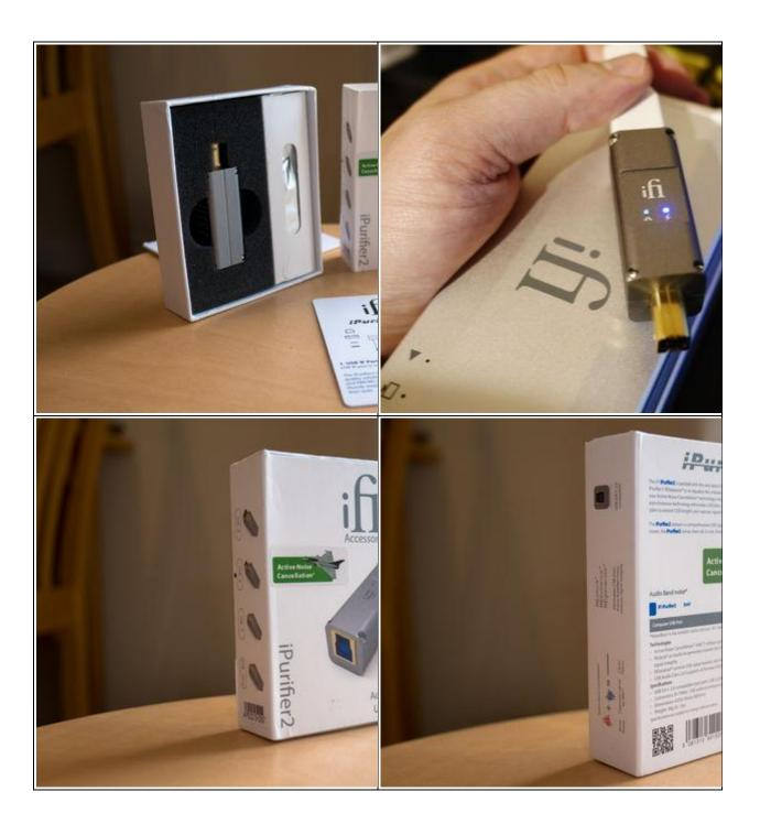
The iPurifier2 has two LEDs. When the device is receiving power but not plugged into a DAC both lights are blue. Plug the iPurifier2 into a DAC and the left light turns green.
