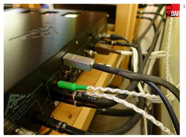
applied two tweaks to the Babyface: vibro-absorbing material on all internal chips and capacitors and a cable that took 15-pin VGA (output of Babyface) to male XLR connectors via 6 feet Canare L-4E6S.
